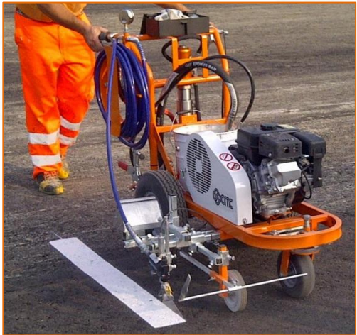
Removable paint gun to use as manual gun (for stenciling) or as automatic gun (for line)
